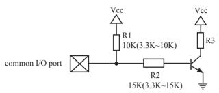
If I/O is configed as "weak" pull-up, you should add a external pull-up resistor R1(3.3K~10K ohm). If no pull-up resistor R1, proposal to add a 15K ohm series resistor R2 at least or config I/O as "push-pull" mode.
