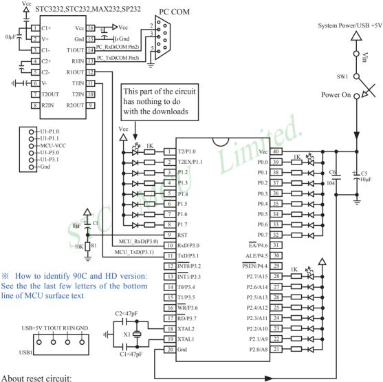
When the crystal frequency X1 is 4MHz, capacitors C2 and C3 should all be 100pF.
