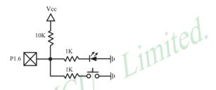
It can save a lot of I/O ports that STC89C51RC/RD+ MCU I/O ports can used as the LED drivers and key detection concurrently because of their feature which they can be set to the weak pull, the strong pull (push-pull) output, only input (high impedance), open drain four modes.
