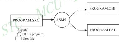
Figure 1 Assembling a source program
