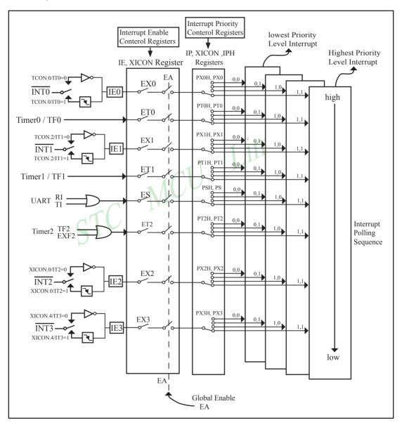
Figure STC89C51RC/RD+ series Interrupt Structure diagram
