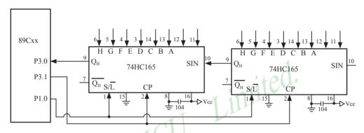
74HC165 is a 8-bit parallel input shift register, when S/L (Shift/Load) pin is falling to low level, the parallel port data is read into internal register, and now, if S/L is raising to high and ClockDisable pin (15 pin) is low level, then clock signal from CP pin is enable. At this time register data will be output from the Dh pin (9 pin) with the clock input.
