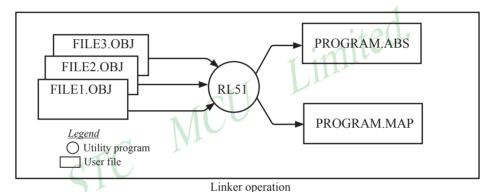
As relocatable modules are combined, all values for external symbols are resolved with values inserted into the output file. The linker is invoked from the system prompt by
