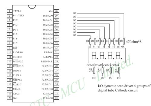
Maximum output current sunk by P0 ports pins of STC89C51RC/RD+ series 5V MCU is 12mA, and the other ports pins' is 6mA.
