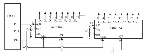
When serial port is working in MODE0, the serial data is input/output from RXD(P3.0) pin and serial clock is output from TXD(P3.1). Serial data is always starting transmission from the lowest bit.
